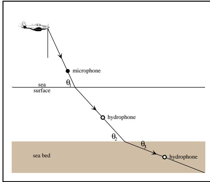
Fig. 5. Schematic showing refraction of a ray through a three layered, horizontally stratified environment.
