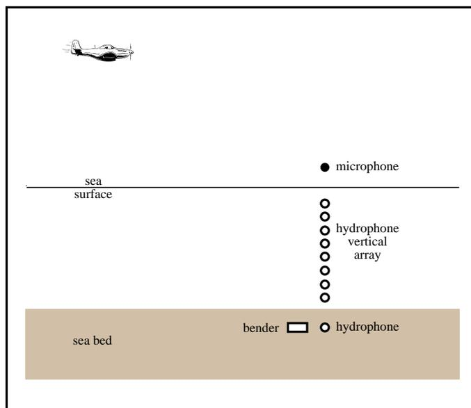
Fig. 2. Schematic of sensor configuration at station B for the experiment of 2 July 2002. The buried bender and hydrophone were 75 cm beneath the seawater-sediment interface and the microphone was 1 m above the sea surface.
