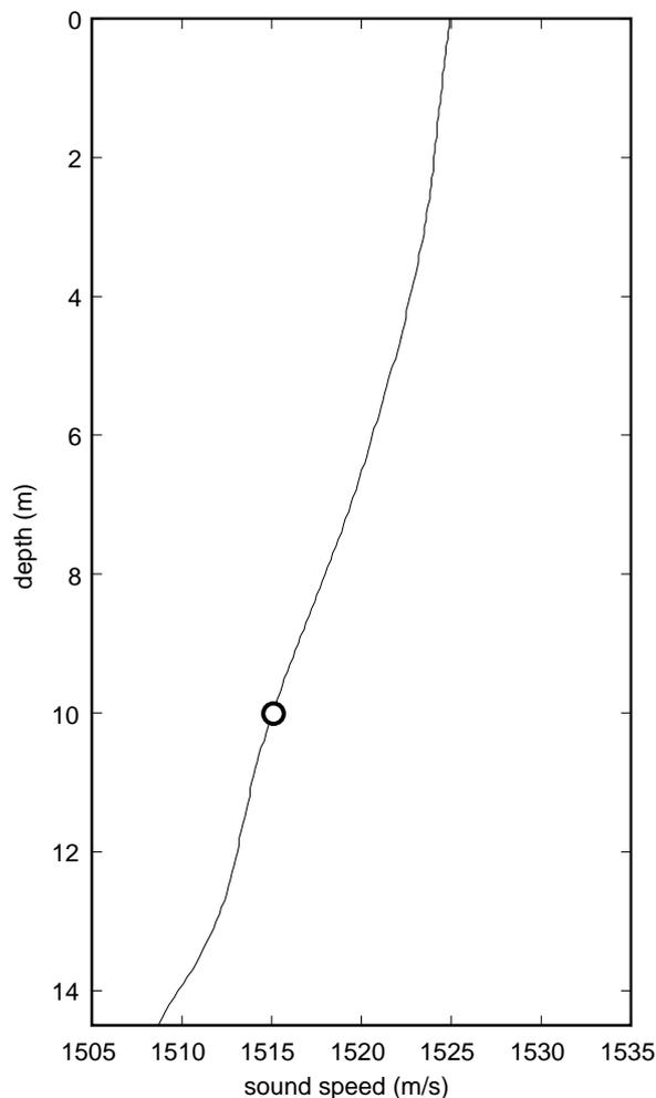
Fig. 7. Sound speed profile in water column, as measured during the experiment of 2 July 2002. The profile was determined from the average of four casts of a Sea-Bird temperature profiler, with smoothing applied using a curve-fitting routine. The small circle identifies the depth of the hydrophone that returned the spectrogram in Fig. 4(b).
