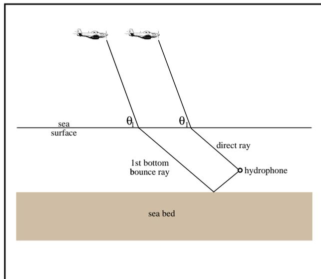
Fig. 8. Direct and first-bottom-bounce arrivals as the aircraft approaches a hydrophone, assuming total reflection at the sea bed. Both rays have the same launch angle and hence identical Doppler-shifted frequencies.
