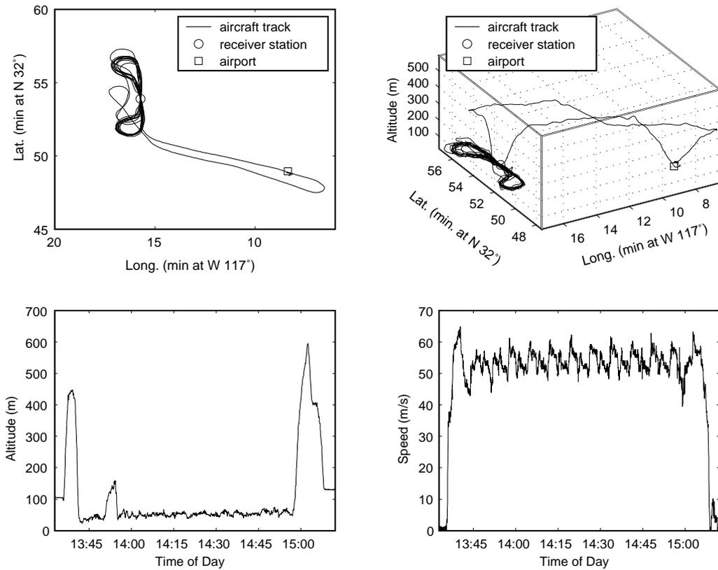
Fig. 3. GPS flight data for the experiment of 2 July 2002. Clockwise from top left, the panels show lateral position, 3-D track, ground speed versus time and altitude versus time. Total flight time from take-off to landing was 1.7 hours.
