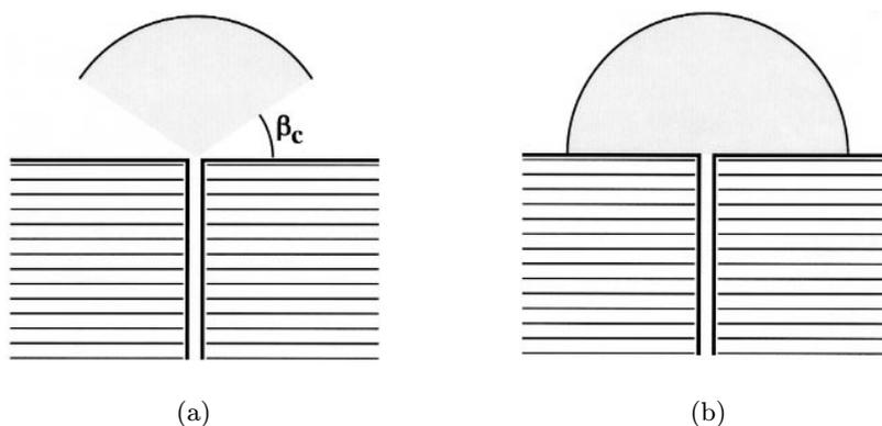
Fig. 3. Sketch depicting the distribution (shading) of high-frequency sound in the atmosphere. (a) Fast magma: no acoustic energy propagates at elevation angles less than  $\beta_c$ ; (b) Slow magma: acoustic energy is essentially uniformly distributed through all elevation angles between 0 and  $\pi/2$ .
