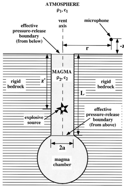
Fig. 1. Axi-symmetric (2-D) model of the magma column and atmosphere used in the analysis. Density,  $\rho$ , and sound speed,  $c$ , are taken to be constant in the atmosphere and magma, denoted by subscripts 1 and 2, respectively.
