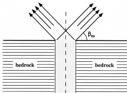
Fig. 2. High-frequency, parallel, parallel-sided beam of sound (arrows) associated with the  $m$ th mode radiating into the atmosphere.
