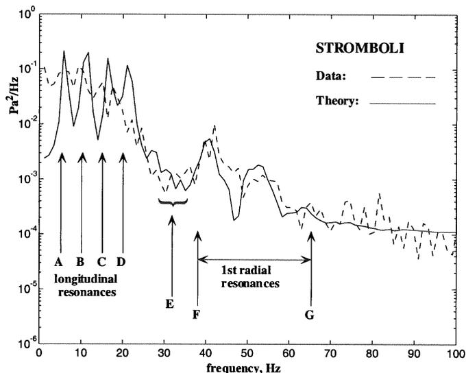
Fig. 5. Spectrum (measured and theoretical) of the airborne sound from an explosive event at Stromboli.
