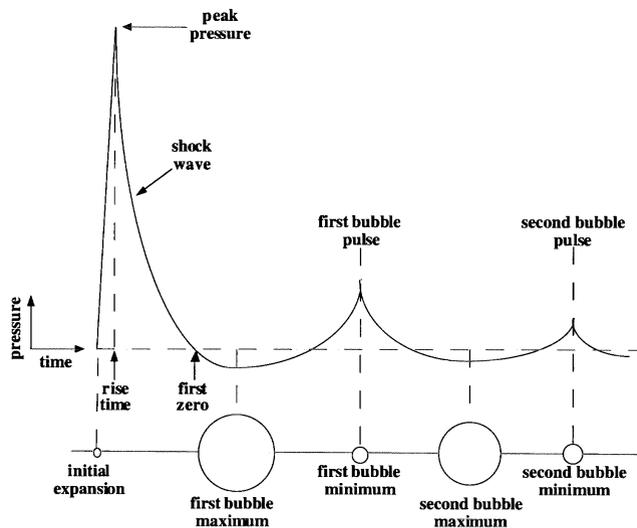
Fig. 4. Gas bubble oscillations in the magma column and the associated pressure waveform.
