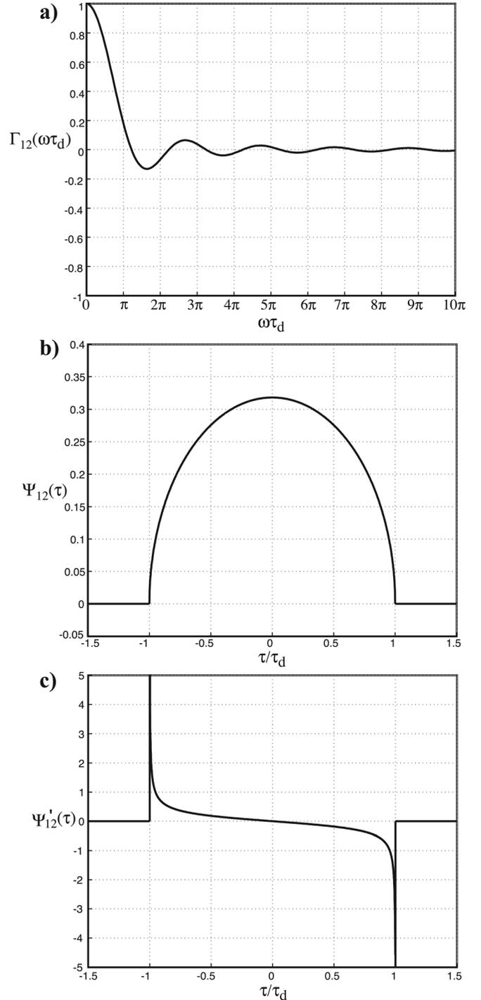
FIG. 10. Deep-water noise and horizontally aligned sensors: (a) coherence function from Eq. (36); (b) normalized cross-correlation function from Eq. (38a); (c) its derivative with respect to delay time from Eq. (38b).
