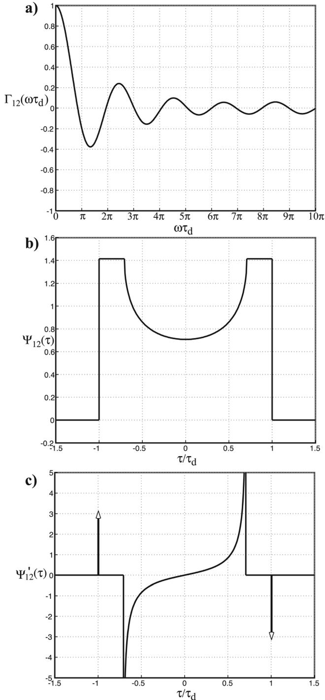
FIG. 5. Horizontal noise lobe,  $\gamma = \pi/4$ , and horizontally aligned sensors: (a) coherence function computed from Eq. (21); (b) normalized cross-correlation function from Eq. (24a); (c) derivative of the normalized cross-correlation function from Eq. (24b).
