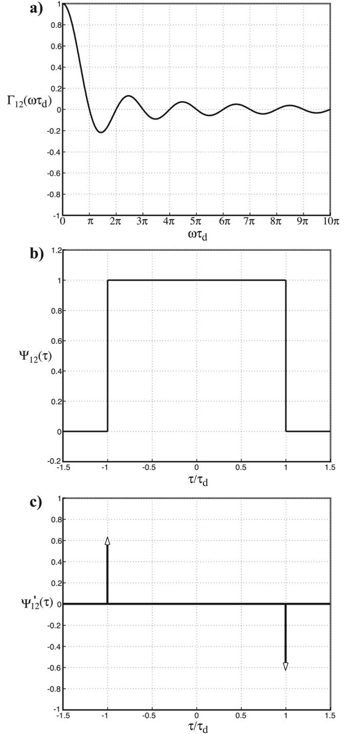
FIG. 2. Isotropic noise: (a) coherence function evaluated from Eq. (17a); (b) normalized cross-correlation function from Eq. (17b); (c) derivative of the normalized cross-correlation function with respect to delay time from Eq. (17c) (open arrows represent delta functions).
