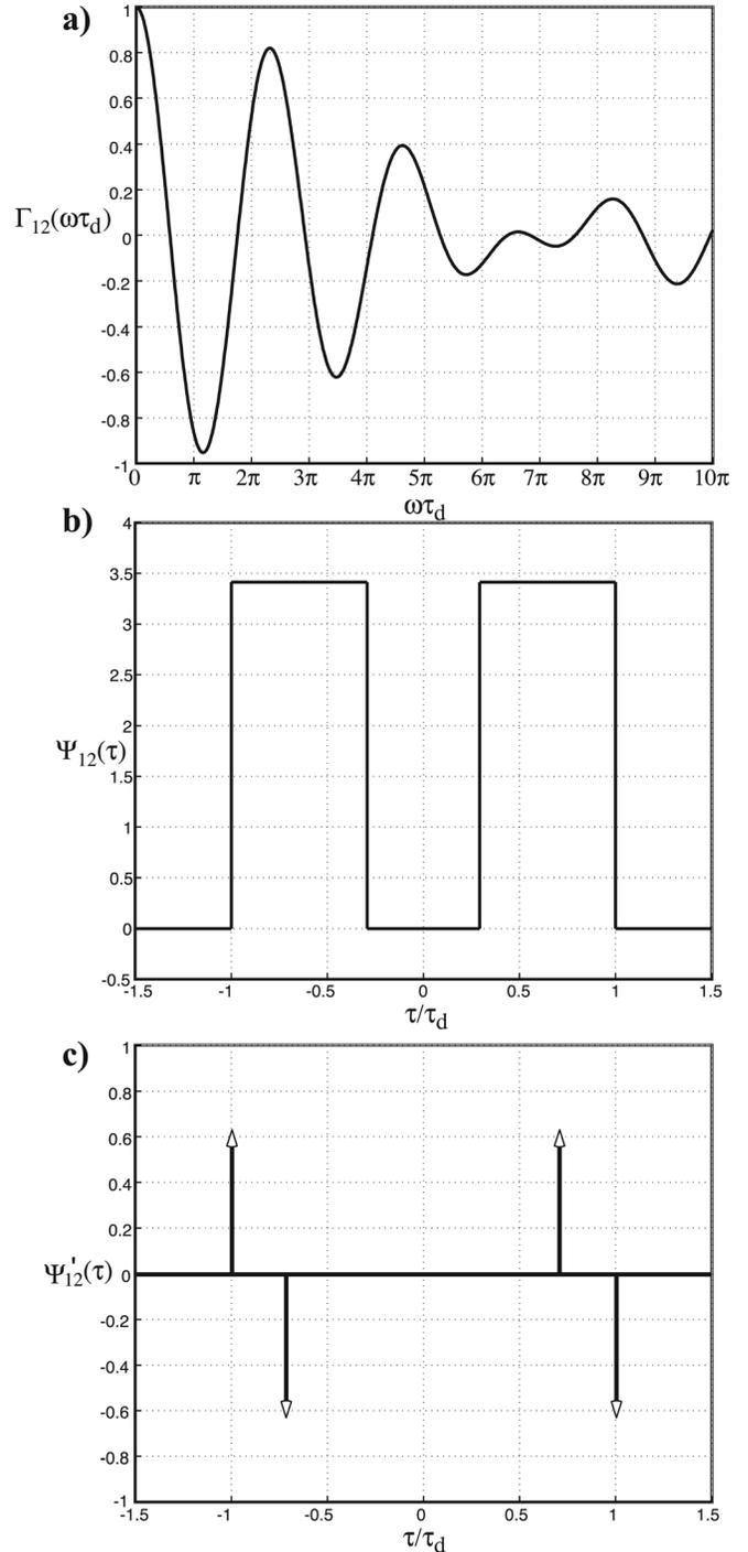
FIG. 7. Horizontal noise notch,  $\beta = \pi/4$ , and vertically aligned sensors: (a) coherence function evaluated from Eq. (26a); (b) normalized cross-correlation function from Eq. (26b); (c) derivative with respect to time delay of the normalized cross-correlation function, from Eq. (26c).
