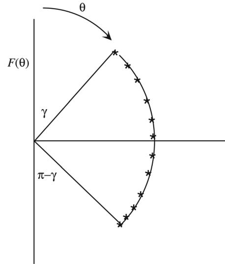
FIG. 3. Directional density function showing a horizontal noise lobe generated by distant sources distributed uniformly (statistically) over the interval  $\gamma \leq \theta \leq (\pi - \gamma)$ .
