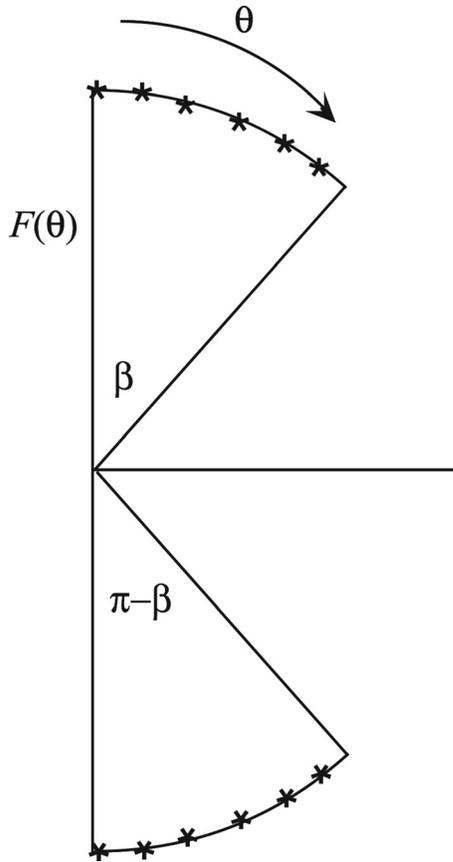
FIG. 6. Directional density function showing noise notch, symmetrical about the horizontal and extending over the interval  $\beta \leq \theta \leq (\pi - \beta)$ , with uniformly distributed noise on either side.
