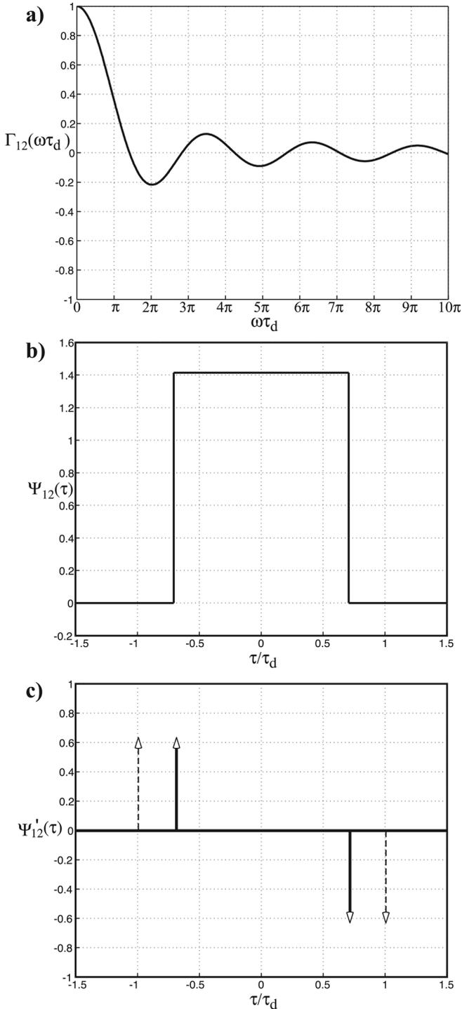
FIG. 4. Horizontal noise lobe,  $\gamma = \pi/4$ , and vertically aligned sensors: (a) coherence function, evaluated from Eq. (20a); (b) normalized cross-correlation function, evaluated from Eq. (20b); (c) schematic showing the delta functions in Eq. (20c) (solid open arrows) and the Greens functions,  $g_{12}(-t)$  and  $-g_{12}(t)$ , in Eq. (18b) (dashed open arrows).
