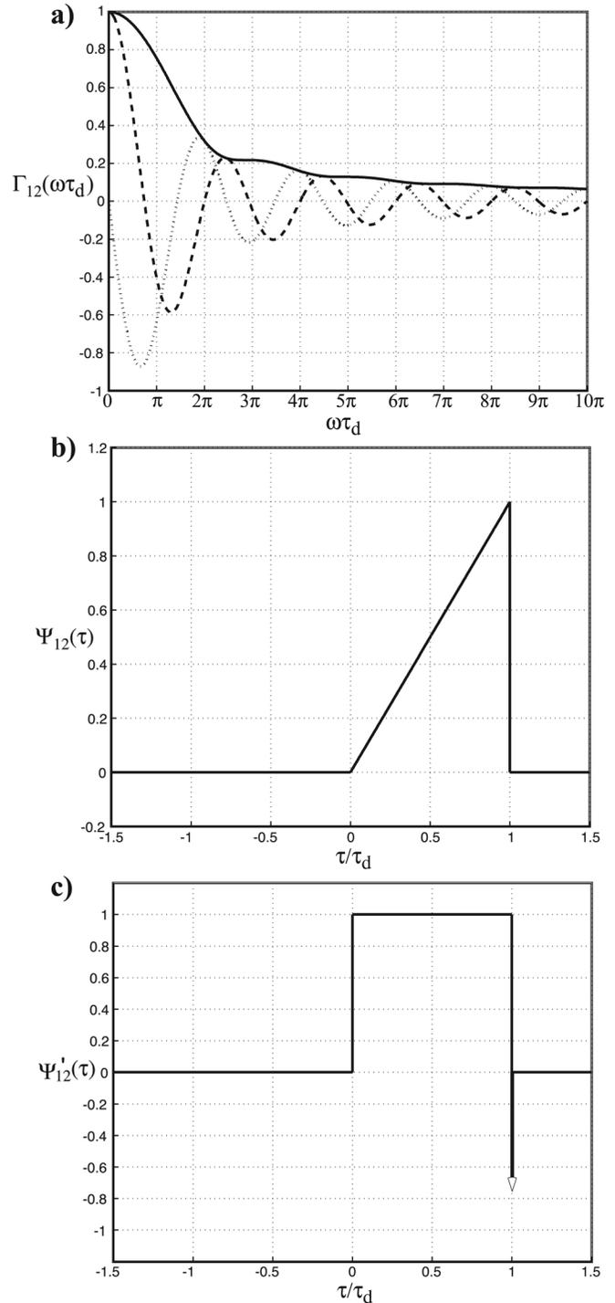
FIG. 9. Deep-water noise and vertically aligned sensors: (a) real (dashed line), imaginary (dotted line), and absolute value (solid line) of the coherence function from Eq. (31); (b) normalized cross-correlation function from Eq. (33b); (c) its derivative with respect to time delay from Eq. (34).
