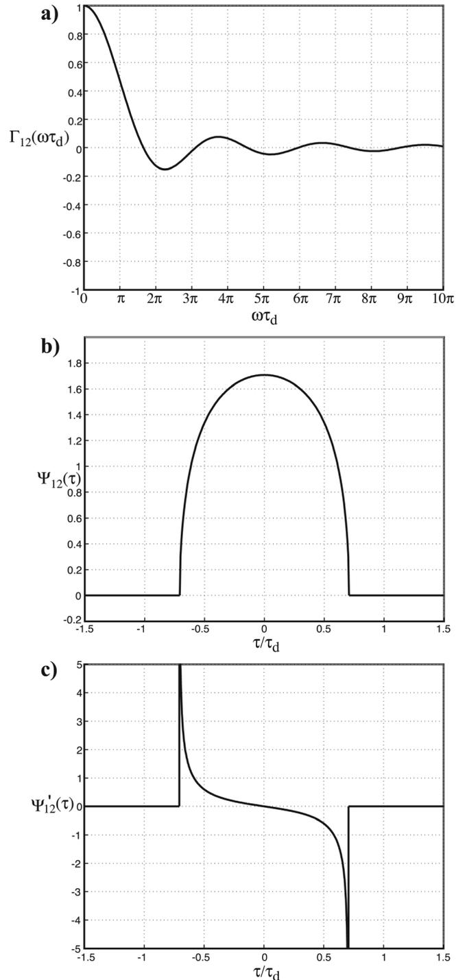
FIG. 8. Horizontal noise notch,  $\beta = \pi/4$  and horizontally aligned sensors: (a) coherence function evaluated from Eq. (27b); (b) normalized cross-correlation function from Eq. (28); (c) derivative of the normalized cross-correlation function from Eq. (29b).
